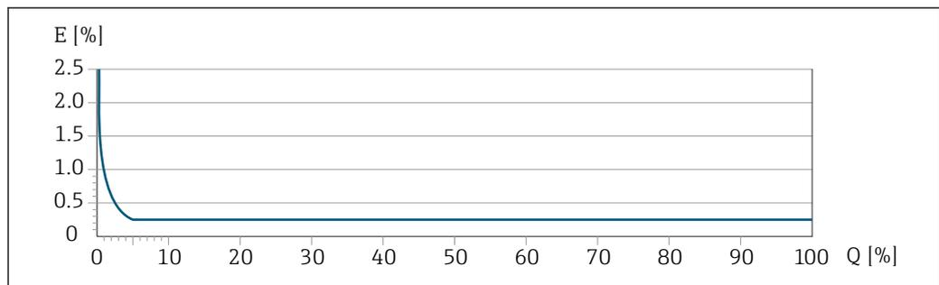
E Maximum measured error in % o.r. (example: DN 25)
