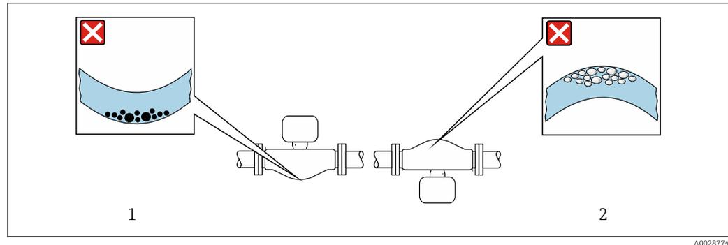
☒ 9 Orientation of sensor with curved measuring tube
